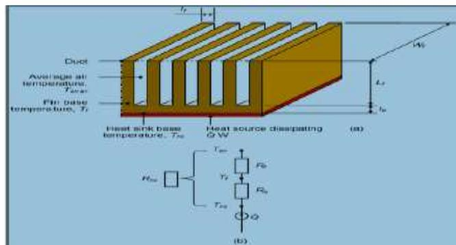
$$q = \frac{T_b - T_\infty}{R_{base} + R_{f,o}}$$
