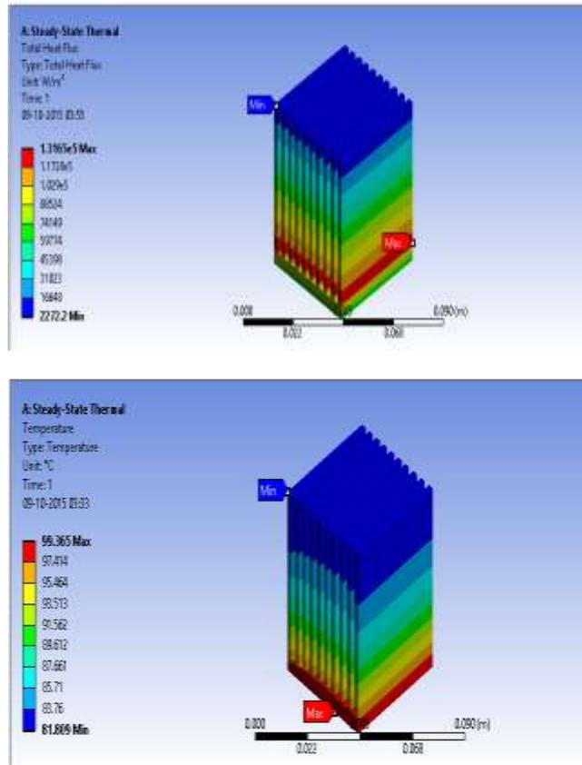
From the above plot it is observed that maximum and minimum temperatures on the heat sink.
